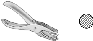
Figure 43: 1/4" Diameter Fiberglass Disk Filters
